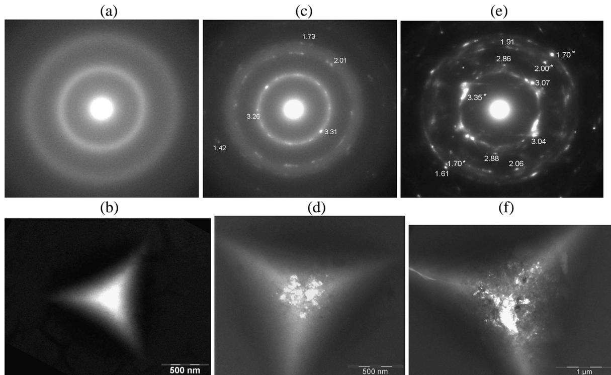
**Figure 1** : Electron diffraction patterns (a,c,e), bright field (b) and dark field (d,f) images of indent sites realised in a 0.3 $\mu\text{m}$  thick amorphous Ge film deposited on GaAs. Indents under 5 mN show no evidence of phase transformation (a,b), the film remains perfectly amorphous. When the maximum load is increased to 10 mN (c,d) crystallites appear with the Ge-I cubic phase. For a 50 mN load, Ge-I and Ge-III (tetragonal or ST-12) phases are detected [2].
