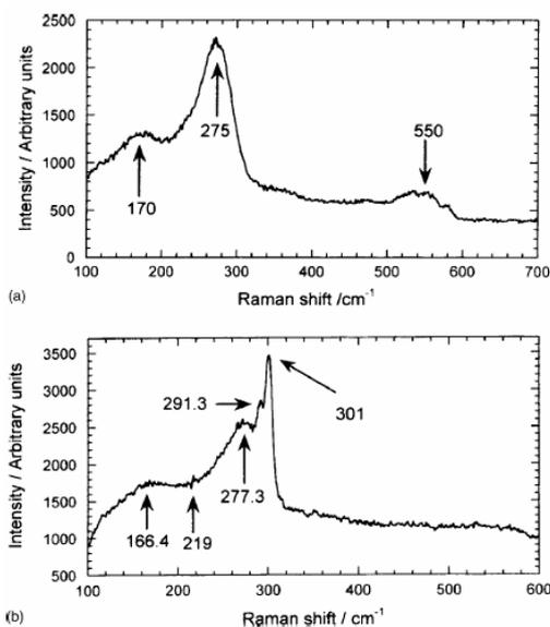
**Figure 2** : Raman spectra of (a) the pristine 0.3  $\mu\text{m}$  thick amorphous germanium film and (b) a 53 mN residual Vickers diamond indentation in the amorphous Ge film. Note that the indentation causes a dramatic change in the Raman spectrum. The sharp peak at 301  $\text{cm}^{-1}$  is the same as that of a pristine Ge-I single crystal (not shown) [2].
